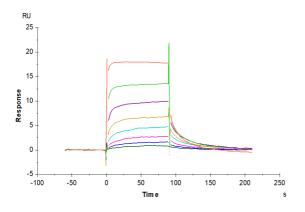
Human FcRn, His Tag captured on CM5 Chip via anti-his antibody can bind Human IgG1 Fc, No Tag with an affinity constant of 0.28  $\mu$ M as determined in SPR assay (Biacore T200).
