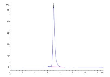
The purity of Human IgG1 Fc is greater than 95% as determined by SEC-HPLC.
